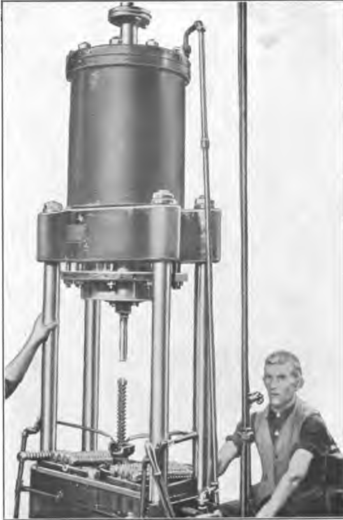
FIG. 65.—Broaching on a 20-ton Watson-Stillman press.
